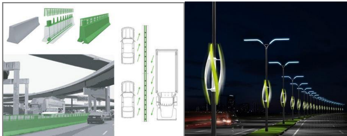
Figure 7: Examples of wind generation systems that harness air movement from passing traffic
