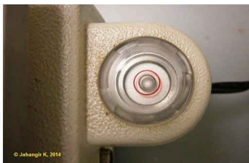
Correctly centred balance (bubble in middle of circle)
