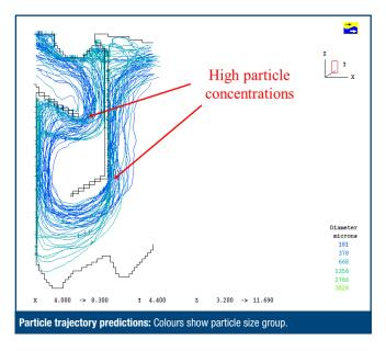
CFD has been used to modify this and many other convection bank designs so that peak velocities are lower and cross flow is increased. Lower peak velocities reduce tube wear and more cross flow increases heat transfer.
