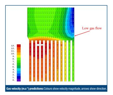
CFD has been used to evaluate boiler design modifications such as the introduction of a furnace exit baffle as seen in the gas velocity and particle trajectory plots below.
