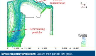
A furnace exit baffle helps promote recirculation of gas and particles down the front wall of the furnace which should improve burnout. However it could also cause the gas and particle flows to be concentrated towards the top of the convection bank, affecting heat transfer and tube wear.
