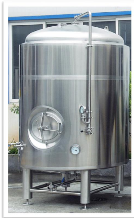
Figure 4. Cold liquor tank
