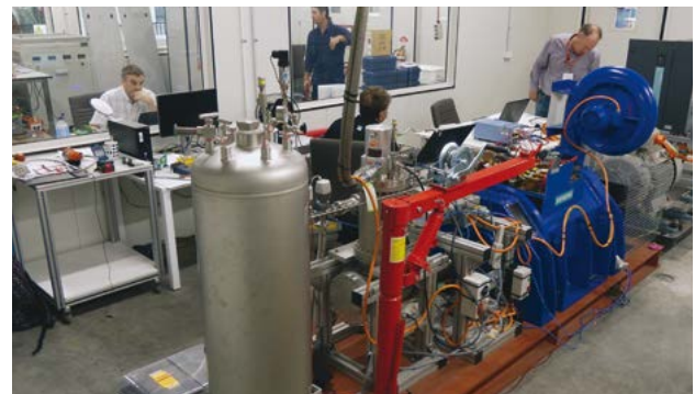
Preliminary testing and commissioning of the HTS1 superconducting synchronous machine at Banyo Pilot Plant Precinct.
