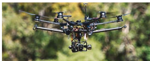
UAV in flight with thermal camera during UAV operations at Pimpama.
