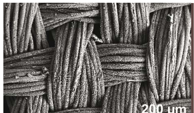
A scanning electron microscopy image shows the nanoscale features on the individual fibres of the fabric.
