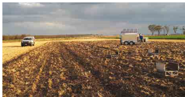
Researchers using an automated solar-powered sampling system to measure soil-borne greenhouse gas fluxes at Felton, in south-east Queensland
