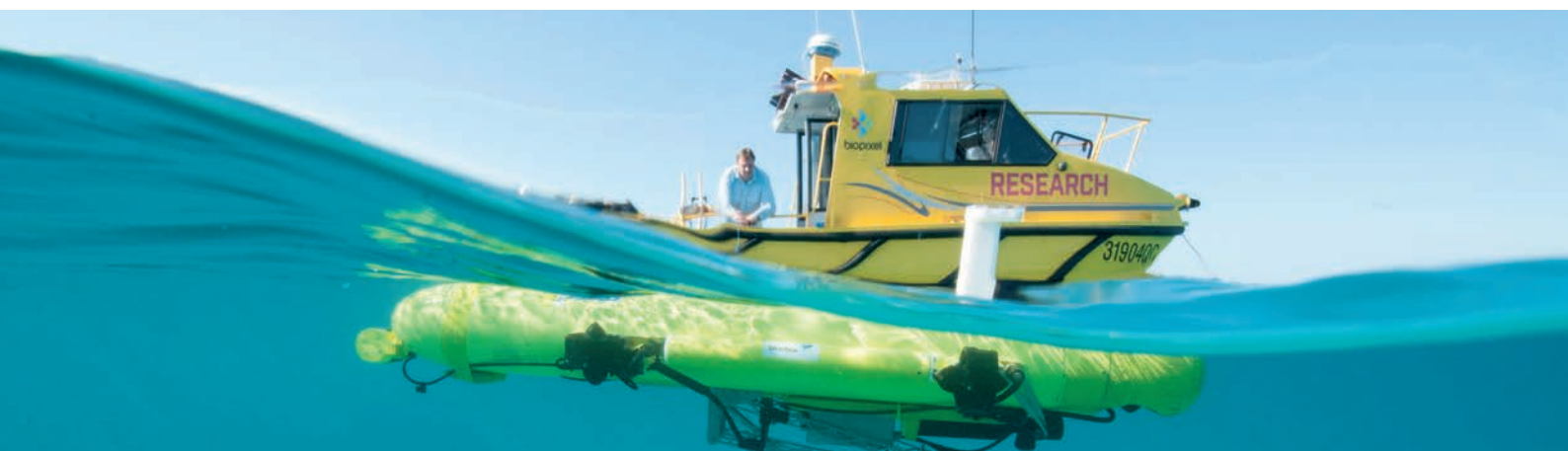
COTSbot, an underwater robot developed by Dr Matthew Dunbabin (on the boat) and Dr Feras Dayoub to autonomously detect and control crown-of-thorns starfish (COTS) on the Great Barrier Reef
