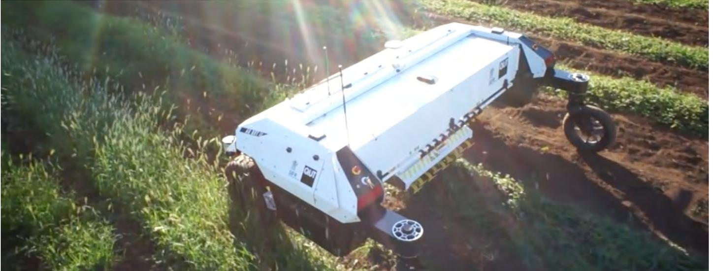
QUT is working on small, lightweight robots that are part of a new generation of agricultural machines. These robots are designed for getting rid of weeds, applying vital nutrients to crops, and gathering data to help farmers make informed decisions about their crops.
